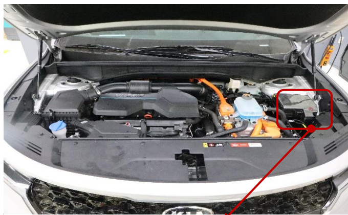
Engine room fuse box
