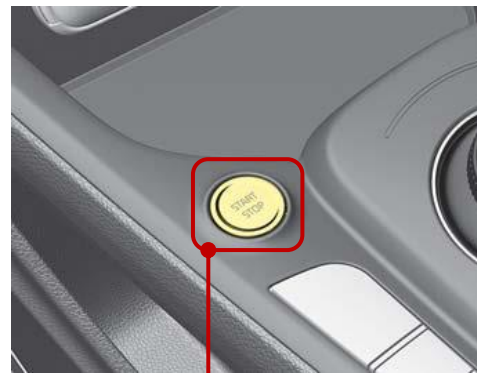
Pulsante "POWER" START/STOP
