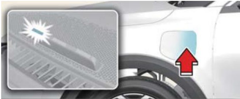
Operation of charging indicator lamp
