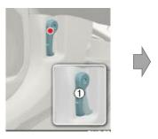
1. Pull the release lever(1) to unlatch the hood. The hood should pop open slightly.
